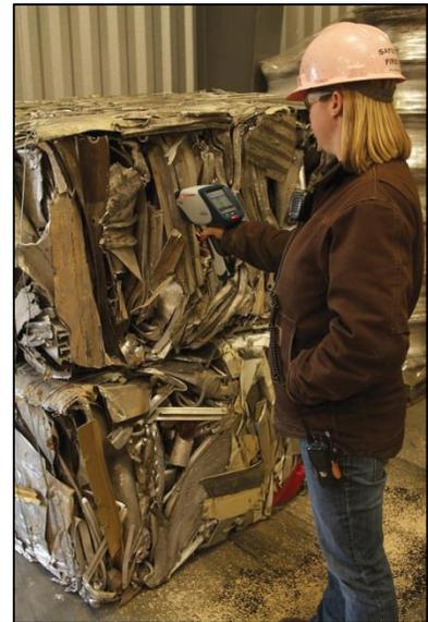
Figure 3: Metal sorting by means of handheld XRF
