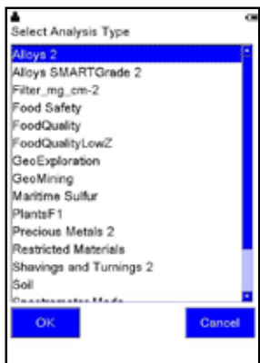
Factory ready calibrations are available to enable point-and-shoot analysis for a variety of applications.
