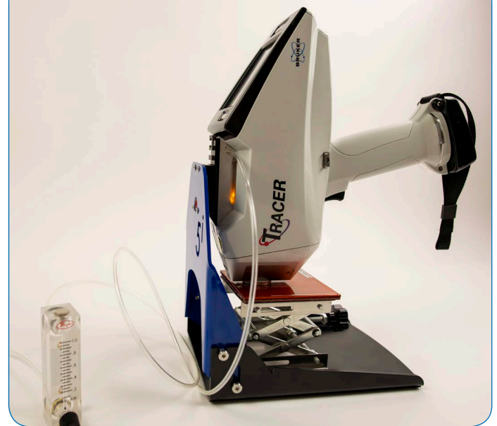
Figure 2: TRACER 5i in nose-down configuration
