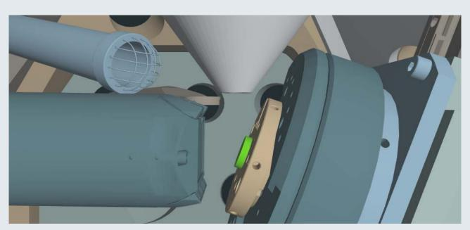
TESCAN Essence™ 3D Collision Model with custom-integrated 3<sup>rd</sup> party EBSD camera intercepts potential collisions of the sample with the camera\*
